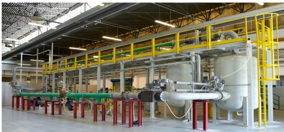
LOCPOWER energy harvesting valve during a flow test in our Valpres facility.
